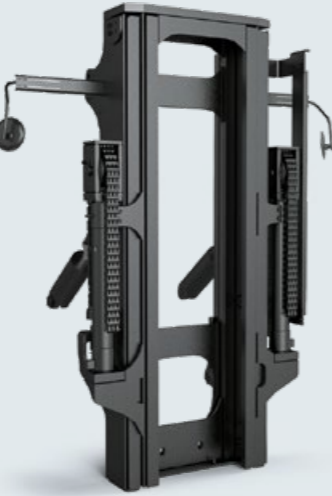
Optional - duplex mast with free lift: Lifting cylinder on duplex mast with free lift positioned to the side of the mast, thus unrestricted view through the central free space of the mast
